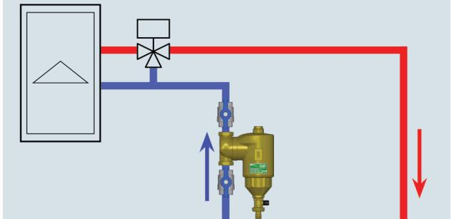
A FAR automatic air vent valve can be installed simply by removing the upper plug and screwing the valve onto the dirt separator. All versions of the dirt separator are available with 1/2" upper connection.
